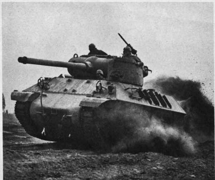
Big, rounded turret and long 90-mm. gun mark the new M-36. Identical with the M-10 ( left ) except for the turret and big gun, its heavier armament should make it even more effective as a tank destroyer.
